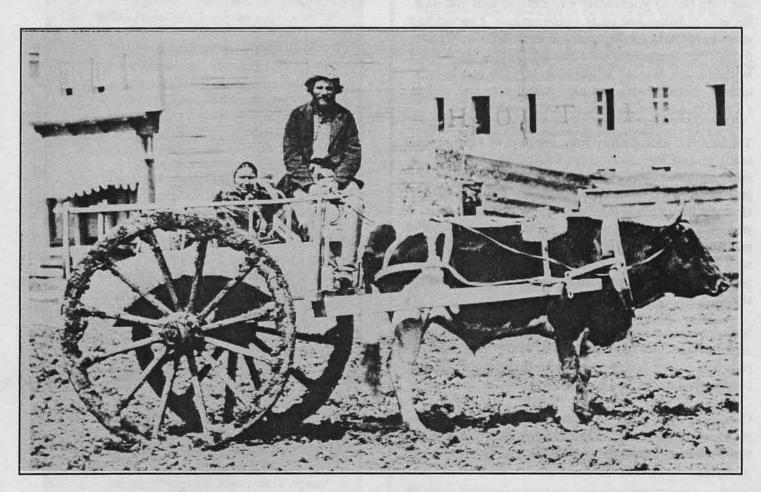
Ox cart on a very muddy Winnipeg street, about 1870. Note the collar around the ox's neck and the leather "tugs' attaching it to the cart shaft ends. Also note the padded "clobber" on the animal's back. A strap running over the clobber supports the weight of the shafts. See story pages 8-10.
