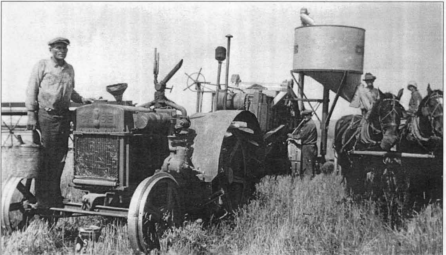
In 1927, the Roen brothers also purchased this Case 18-36 Han-Pan kerosene powered tractor. Here they take a break to refuel and dump grain from the 60 bushel hopper into a horse-drawn grain tank. CCHS Collections.
